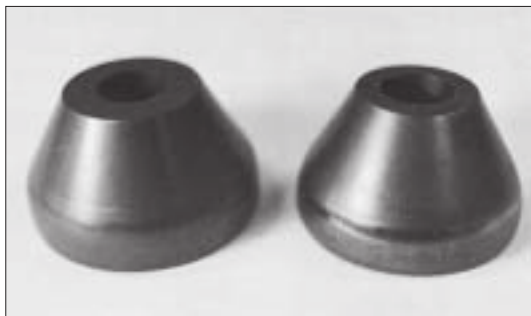
PVD coated tools in Uddeholm Vanadis 23 for cold forming of tubes.
