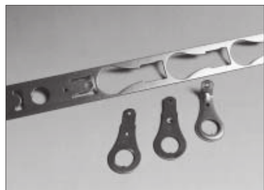
Stainless steel fastener stamped with a Uddeholm Vanadis 23 die and Uddeholm Vanadis 4 punch.
