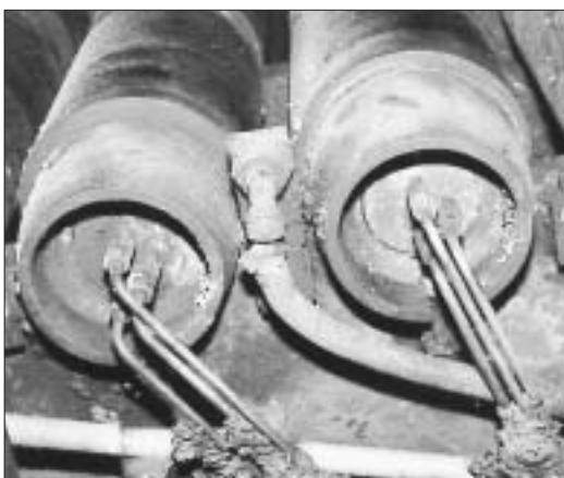
The combination of good high-temperature strength, wear resistance and good machining properties make THG 2000 suitable for use as rolls in continuous casting machines.
