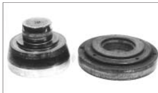
Dies for axial closed die rolling.
