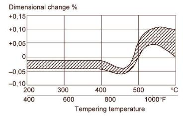
Note: The dimensional changes on hardening and tempering should be added together. The minimum recommended machining allowance is 0.15% per side assuming that stress relief is performed between rough and semifinish machining, as recommended. If not, machining allowances must be increased accordingly.
